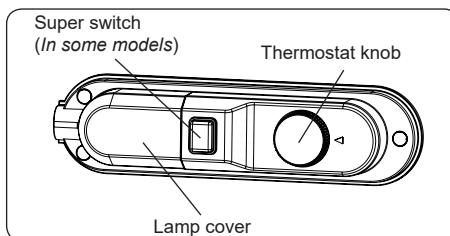
The fridge freezer thermostat automatically regulates the inside temperature of the compartments. By rotating the knob from position 1 to 5, colder temperatures can be obtained.
