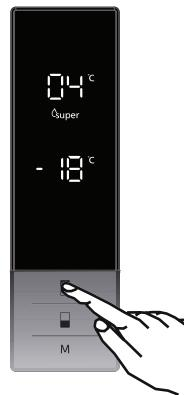
Press cooler set button until super cool symbol will be seen on the screen. Buzzer will sound beep beep. Mode will be set.
