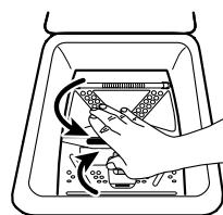
**ATTENTION:** Check that no laundry gets stuck between the flaps, or between flaps and drum. Make sure that the drum flaps are properly locked - depending on the model:
