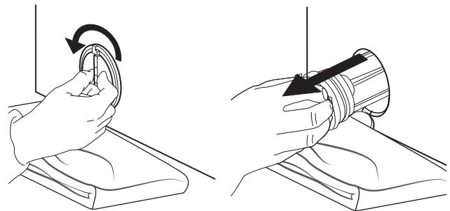
5. Clean the water filter: remove residues in the filter and clean it under running water.
