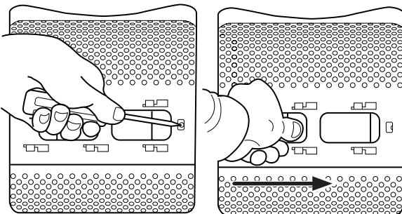
4. Open the drum: you can recover the object through the hole in the drum.
