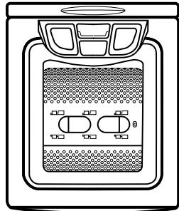
3. Using a screw-driver, press on the plastic end while sliding the blade from left to right. It will fall into the drum.
