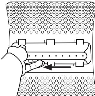
6. Close the drum flaps again, turn the drum through half a turn and check the positioning of the blade at all its anchorage points.
