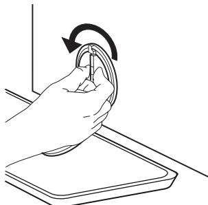
4. Remove filter: Lay a cotton cloth beneath the water filter, which can absorb a small amount of rest water. Then remove the water filter by turning it out anti-clockwise.
