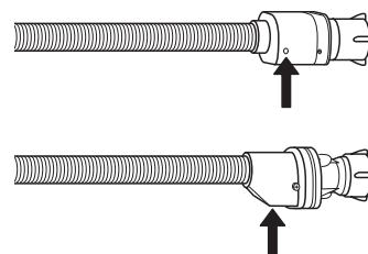
For water stop hoses: check the small safety valve inspection window (see arrow). If it is red, the water stop function was triggered, and the hose must be replaced by a new one. For unscrewing this hose, press the release button (if available) while unscrewing the hose.
