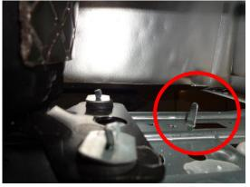
4. Remove first liner of bitumen, then stick to right side of compressor as shown below
